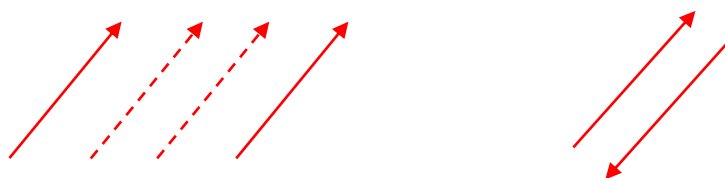
Figure 10 a Representation of vectors by arrows. A vector shifted parallel to itself results in the same vector. b These vectors have the same magnitude but opposite direction.
